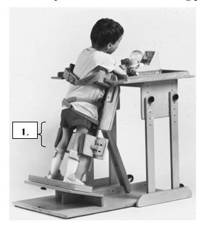
1. Adjust the knee pads. The height of the knee support can be adjusted vertically by removing the corresponding knobs on the back of the stander. Remove the knee support, with the bolts attached, and position to the desired height. Replace the knobs and tighten securely. The width of the lateral support is adjusted by loosening the bolt-knob assembly, sliding the support horizontally, and re-tightening the knob. Note that all kneepads are adjustable with Velcro®-like hook and loop attachments.
