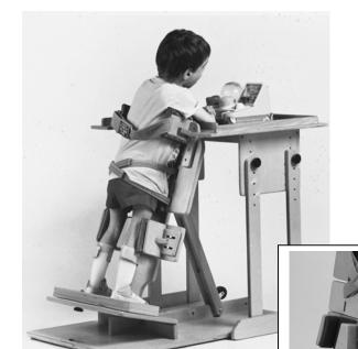
**4. Adjust the pelvic straps.** The pelvic straps are designed to be used in the crossed position, and can be inserted to pull from either side as needed to position the pelvis. To change the position of the straps pull them out through the back of the stander and re-insert in the desired slots.
