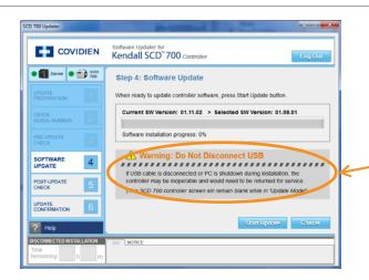
WARNING: Once the "Start Update" button has been selected the Kendall SCD 700 series controller SHOULD NOT be disconnected from the personal computer for the remainder of the update.
