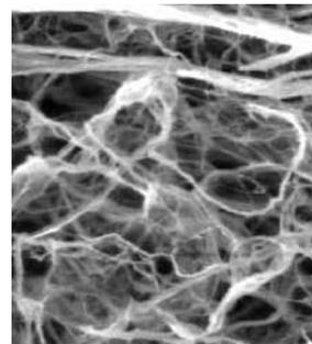
2B. Puracol Plus Native MicroScaffold wound dressing as seen through an electron microscope. The open porous structure increases the internal surface area.
