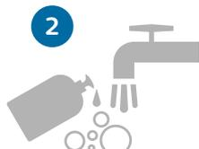
**2** **Chamber:** agitate parts in warm soapy water with liquid detergent for 1 minute then soak for 10 minutes.
