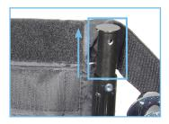
4. Pull upward on seat extension post until the second hole on the seat post lines up with the hole on seat frame. Re-insert screw into bottom hole and turn clockwise to secure in place.
