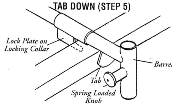
5. Release the spring loaded knob on the Head-end barrel.
