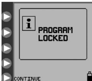
Figure 16. Program Locked screen, which indicates the pump is in LOCK SETTINGS mode.
