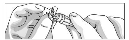
d. Place the new valve cap on the valve.
