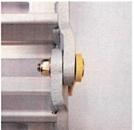
Use the 3/16" Hex Allen Wrench and a 1/2" wrench or the wrench provided. Align ramp sections - insert bolt through hole - tighten with Allen Wrench and wrench provided or a 1/2" socket. **Note:** Do **NOT** fully tighten nut to be able to roll up.
