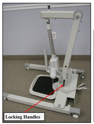
Lifting Actuator is not shown in the figure below to show the tightening of the locking handles.
