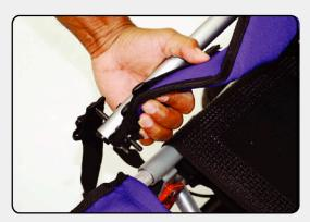
**Step 3a**Remove bolt and pull side frame apart from seat frame, ensure all loose part are in correct sequence before reinserting bolts.
