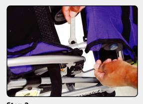
**Step 2**Remove bolts, located on the front of the seat frame in which the telescoping seat depth extension tubes are inserted. Perform on one side at a time. (5/32" Hex Key and 7/16" wrench)
