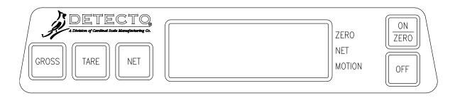
When applying power, make certain the scale platform is empty. Press and hold the **ON/ZERO** key until one of the annunciators (ZERO, NET or MOTION) turn on. When one of the annunciators turn on, release the **ON/ZERO** key. After a second or so the display should indicate a zero weight with the ZERO annunciator turned on. Weighing may now begin. If the display does not indicate zero, press the **ON/ZERO** key again to zero the weight display.
