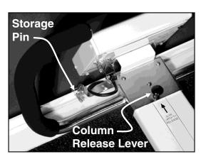
3 Slide the Column Release Lever to release column and lift to full up-right and locked position.
