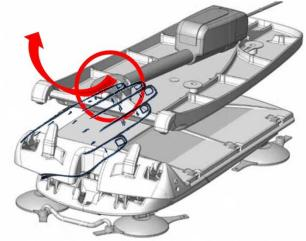
Lift from this part only to remove the backrest from the base of the Aqua Bath Lift.
