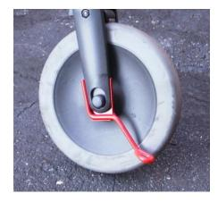
• Remove the center hubcap using a screwdriver or small flat blade.
